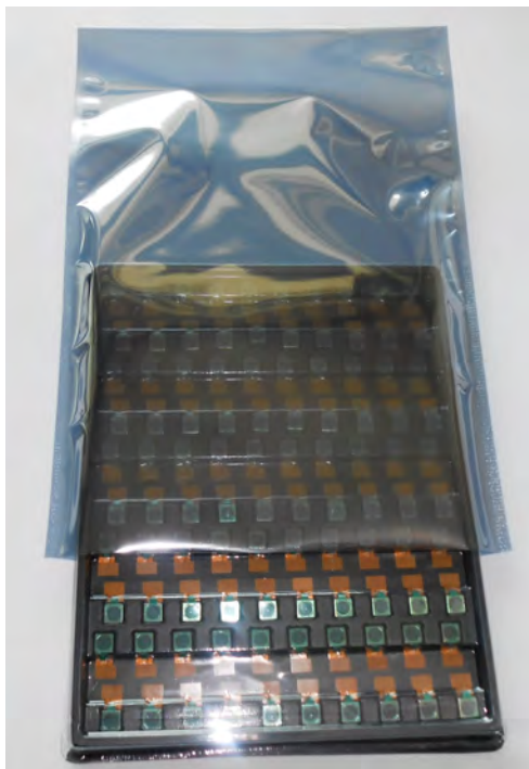
Put Tray into Anti-Static Bag
